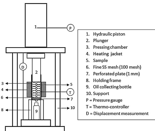
**Fig. 2.** Schematic representation of the hydraulic press.
