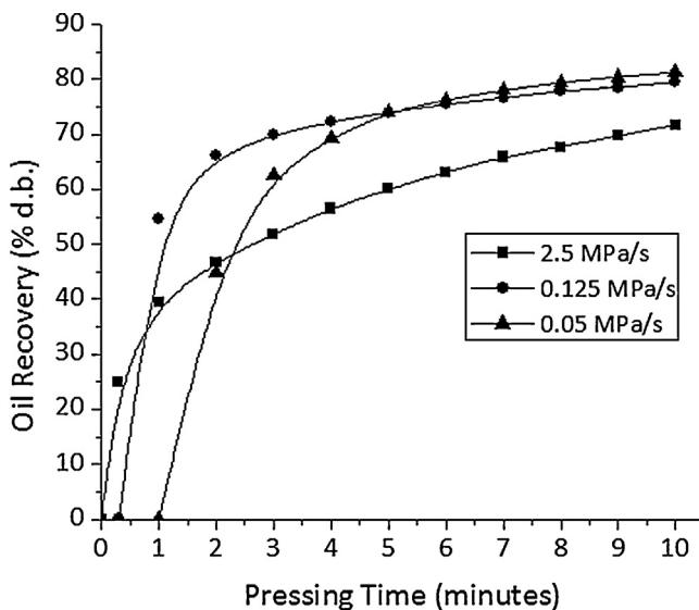
**Fig. 3.** Oil recovery profiles of Jatropha kernels pressed at different compression speeds (moisture content of kernels: 4% (w.b.); applied pressure: 15 MPa; pressing temperature: 60 °C; 10 min pressing).
