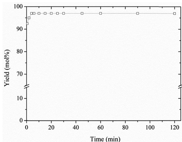
**Figure 4.** FAME yield (mol%) for a typical experiment in a modified CCCS (6:1 molar ratio of methanol to oil, 1%w/w of catalyst concentration, oil flow rate of 16mL/min, methanol flow rate of 4 mL/min, 60°C, 35 Hz).
