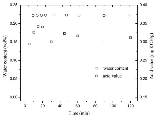
**Figure 9.** Water content (% v/v) and acid value (mg KOH/g) versus time for a FAME refining experiment in a CCCS (FAME flow rate ( $F_{\text{FAME}}$ ): 12 mL/min, Water to FAME flow rate ( $F_{\text{W}}/F_{\text{FAME}}$ ): 0.5, 30 Hz, 50 °C).
