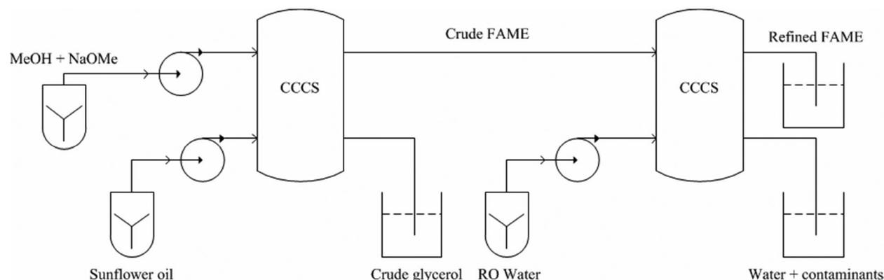
**Figure 10.** Schematic representation of continuous synthesis and refining of sunflower biodiesel in a cascade of two CCCS devices.
