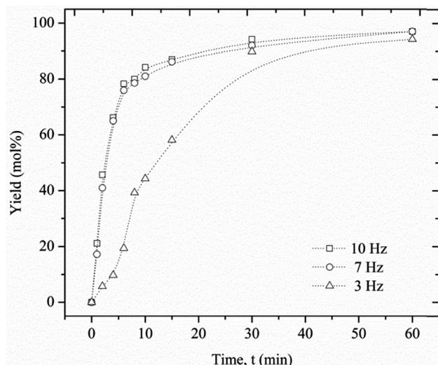
**Figure 3.** Effect of rotational speed on FAME yield in batch (6:1 molar ratio of methanol:oil, 1%w/w catalyst concentration, 20°C).
