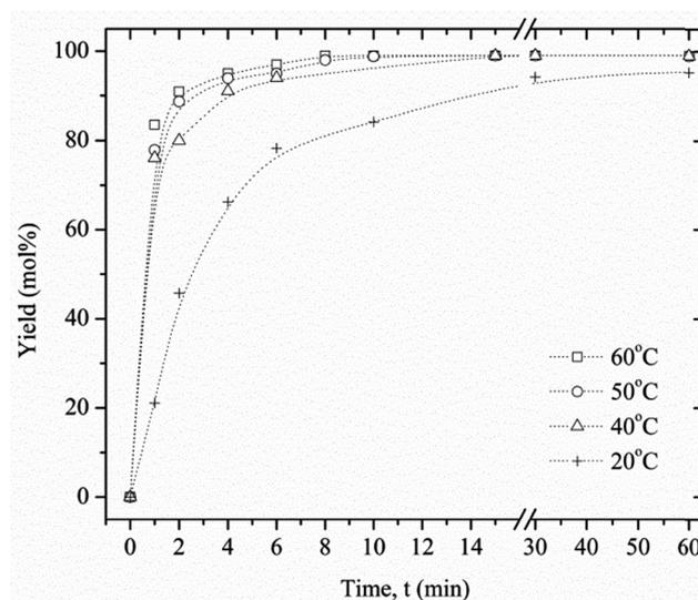
**Figure 2.** Effect of temperature on FAME yield in batch (6:1 molar ratio of methanol:oil, 1%w/w catalyst concentration, 10 Hz).
