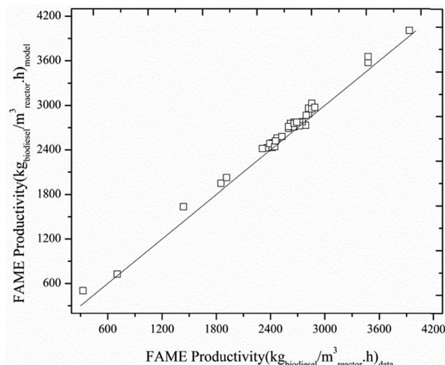
**Figure 7.** Parity plot for the regression model for volumetric FAME production rate.
