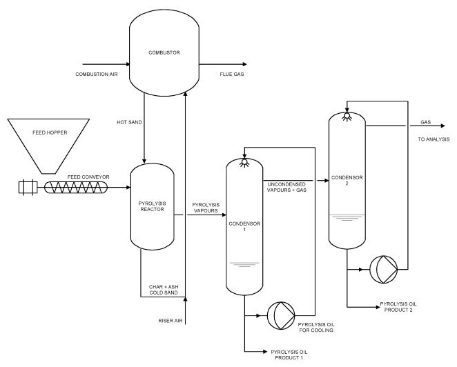
Fig. 4 - Schematic representation of the bench scale flash pyrolysis set-up used in this study.
