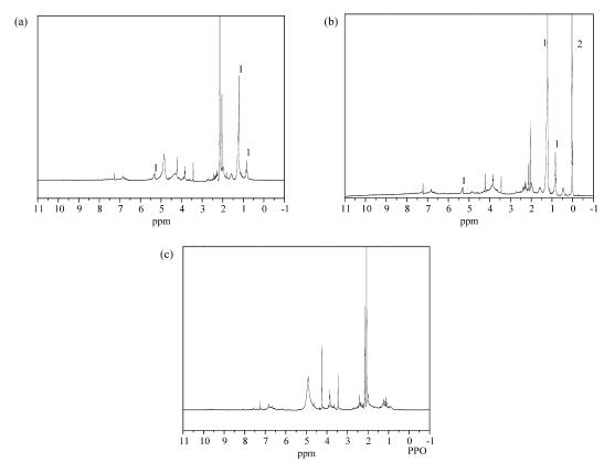
Fig. 5 –  $^1$ H NMR spectra of top (a), middle (b) and bottom (c) sample. (1) Main peaks from PPO; (2) internal standard (tetramethylsilane, TMS). Peak at  $\delta$  7.21 ppm is from the NMR solvent (CDCl<sub>3</sub>). All other peaks are from the various components within a typical pyrolysis oil.
