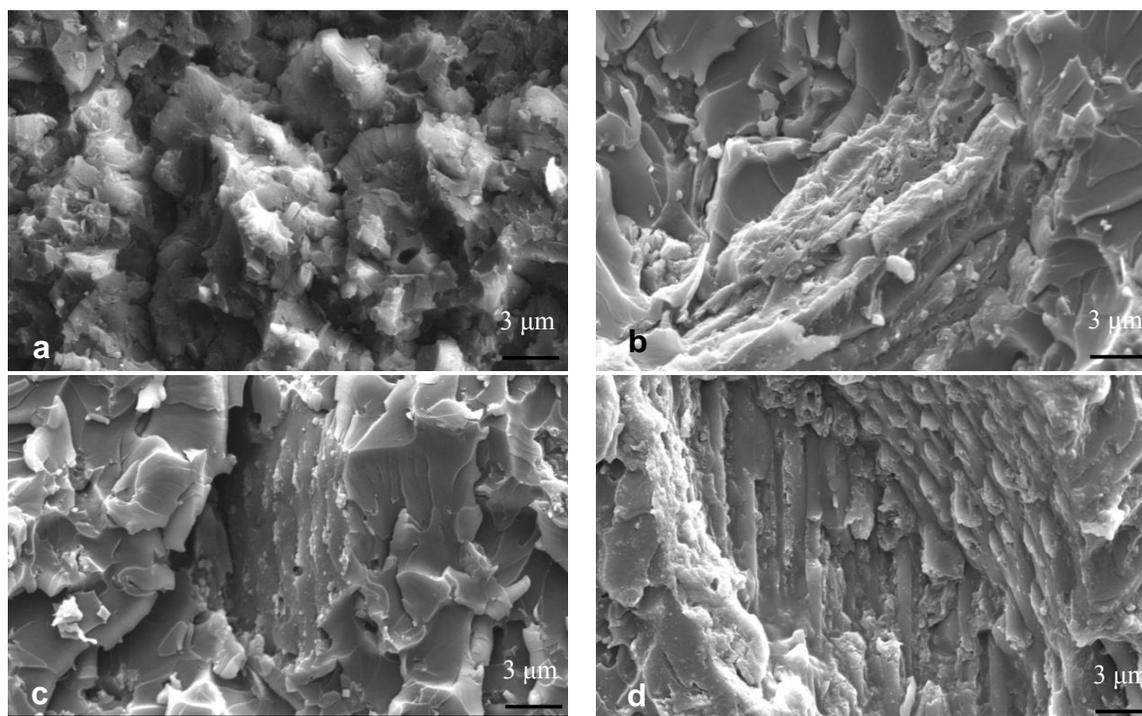
**Fig. 7.** SEM image of the carbon fiber of *Jatropha* seed shell filled vinyl ester composites: (a) Control (source: Sri Aprila *et al.* 2014) (b) after immersion in 5% NaOH for 12 months, (c) after immersion in 5% HCl for 12 months, and (d) after immersion in distilled water for 12 months
