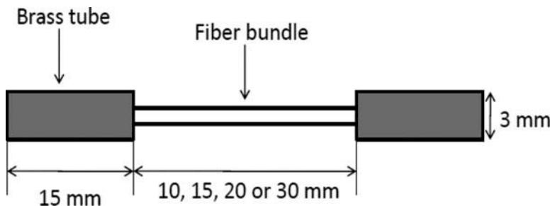
FIGURE 1 Schematic drawing of tensile testing for fiber bundle.
