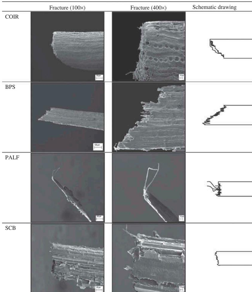
FIGURE 7 Scanning electron micrographs of different types of agricultural residue fibers on fracture surface and their corresponding drawing.
