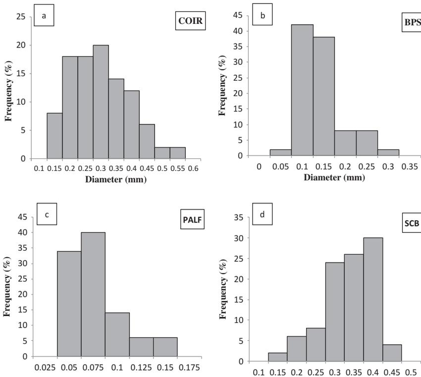
FIGURE 3 Fiber diameter distribution of COIR, BPS, PALF, and SCB fiber (based on 50 readings of each fiber along the length).
