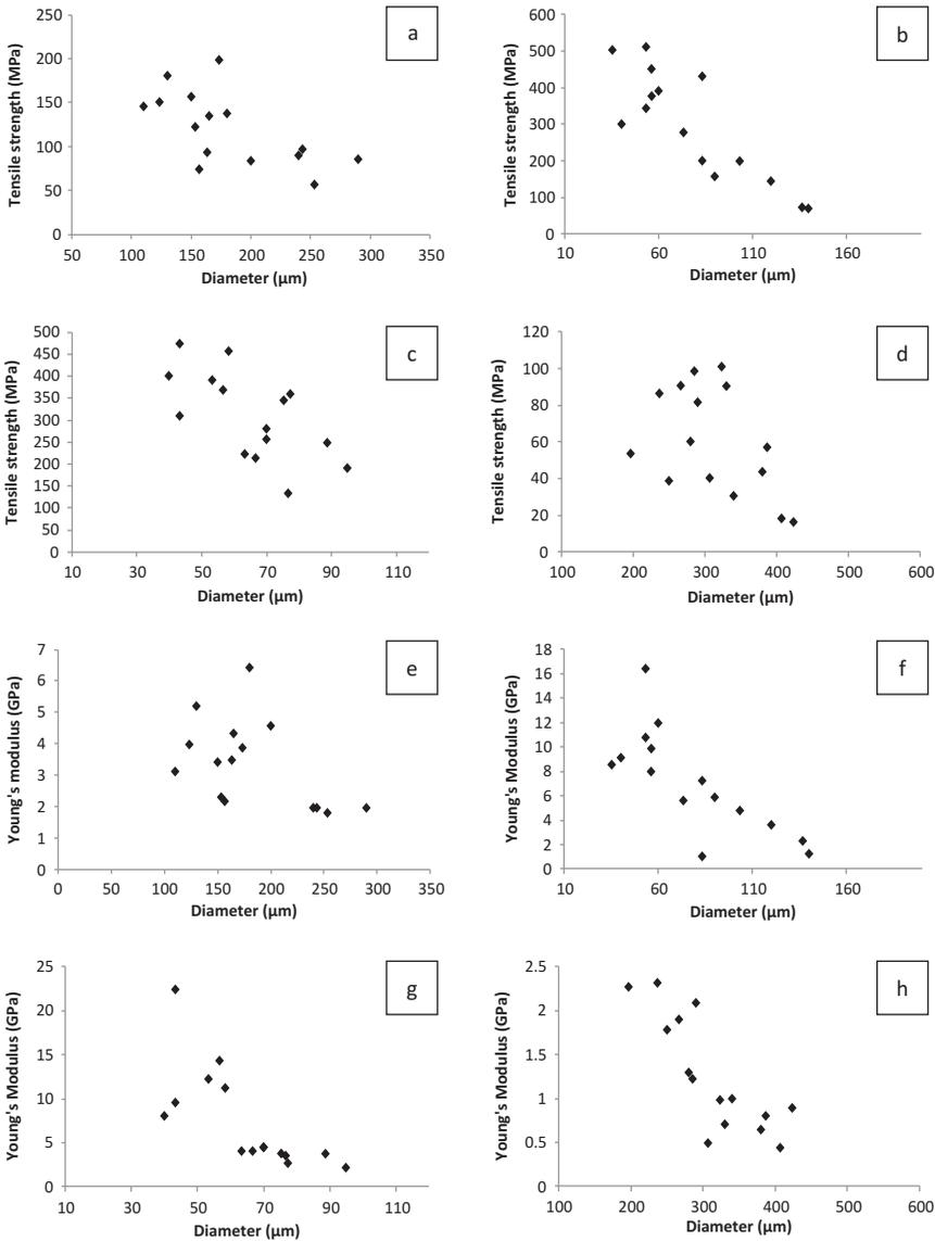
FIGURE 5 Tensile strength and Young's modulus as a function of fiber diameter for COIR (a and e), BPS (b and f), PALF (c and g), and SCB (d and h) at 10 mm gauge length.
