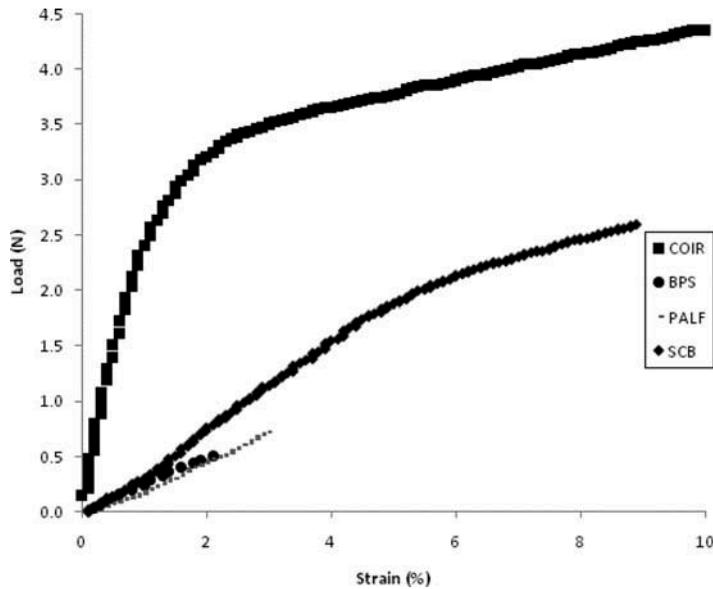
FIGURE 4 Typical load-strain curves of COIR, BPS, PALF, and SCB fiber obtained at a crosshead displacement rate of 20 mm/min.
