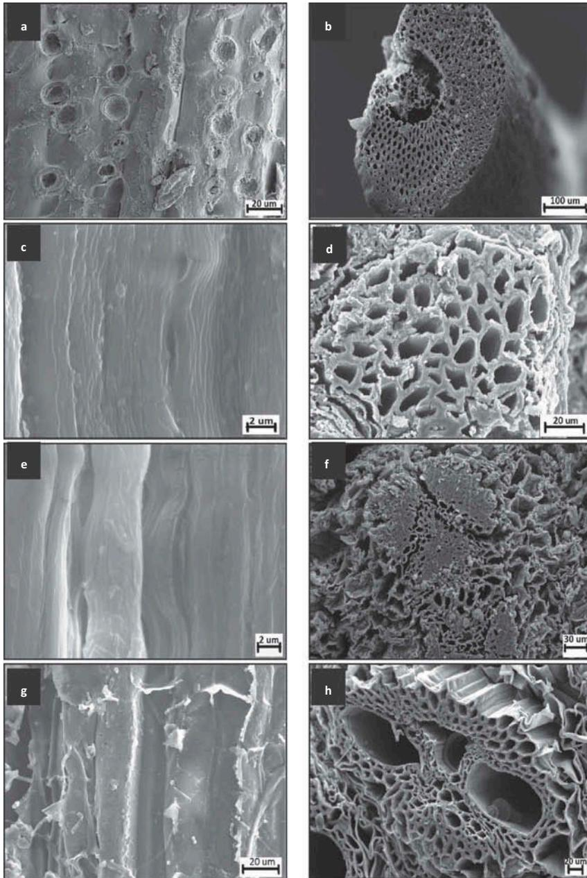
FIGURE 2 SEM micrograph of longitudinal surface of (a) COIR 654 $\times$ , (c) BPS 4670 $\times$ , (e) PALF 4650 $\times$ , and (g) SCB 726 $\times$ , and cross-sectional view of (b) COIR 170 $\times$ , (d) BPS 2050 $\times$ , (f) PALF 297 $\times$ , and (h) SCB 282 $\times$ .
