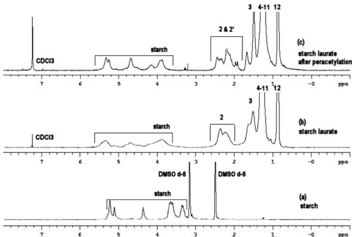
**Fig. 2.** Typical  $^1H$ -NMR spectrum of (a) native starch in  $DMSO-d_6$  at  $60^\circ C$ ; (b) starch laurate, DS = 2.52 (Sample 17, Tab. 1) in  $CDCl_3$  at  $50^\circ C$ ; (c) peracetylated starch laurate, DS = 2.52 (Sample 17, Tab. 1) in  $CDCl_3$  at  $50^\circ C$ . For atom numbering scheme: see Fig. 1.
