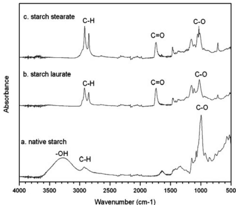
**Fig. 4.** FT-IR Spectra of starch laurate (DS = 2.52, Sample 15, Tab. 1), starch stearate (DS = 2.96, Sample 17, Tab. 1) and native starch.
