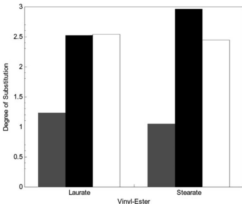
**Fig. 6.** Comparison of DS values with different catalysts (vinyl ester: AHG molar ratio = 3:1, catalyst amount = 2% (w/w), 110°C, DMSO). Gray:  $\text{Na}_2\text{HPO}_4$ ; black:  $\text{K}_2\text{CO}_3$ ; white: Na acetate.
