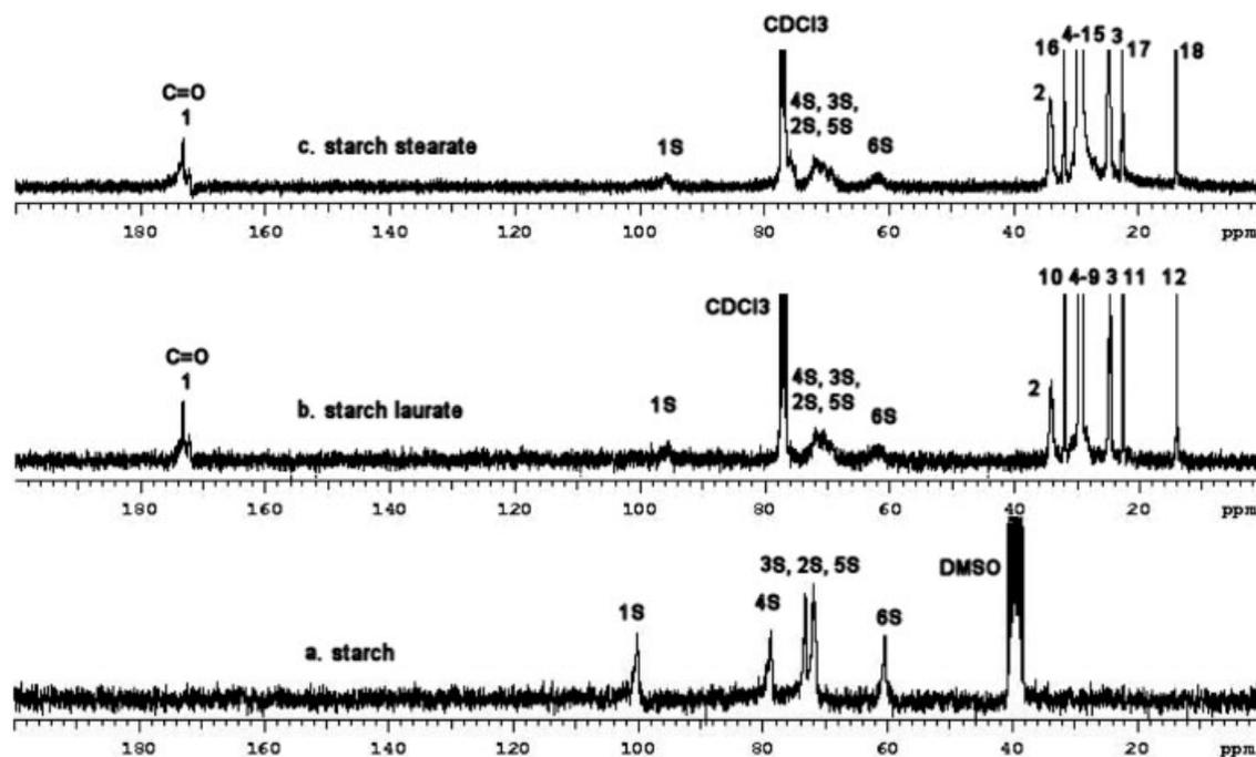
**Fig. 3.** Typical  $^{13}\text{C}$ -NMR spectra of: (a) native starch, in  $\text{DMSO-}d_6$  at  $60^\circ\text{C}$ ; (b) starch laurate, DS = 2.52 (Sample 15) in  $\text{CDCl}_3$  at  $50^\circ\text{C}$ ; (c) starch stearate, DS = 2.96 (Sample 17) in  $\text{CDCl}_3$  at  $50^\circ\text{C}$ . For atom numbering scheme: see Fig. 1.
