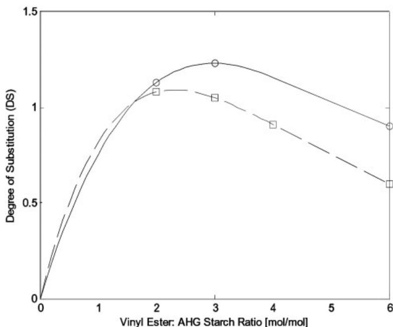
**Fig. 5.** DS of the product as a function of the type of vinyl ester and the vinyl ester: starch ratio (24 h reaction time, 110°C, 2% (w/w) catalyst intake on starch). ○ : starch laurate; □ : starch stearate. Lines for illustrative purposes only.
