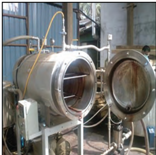
Fig. 1. Impregnation chamber utilized for impregnation of resin in OPTCL.
