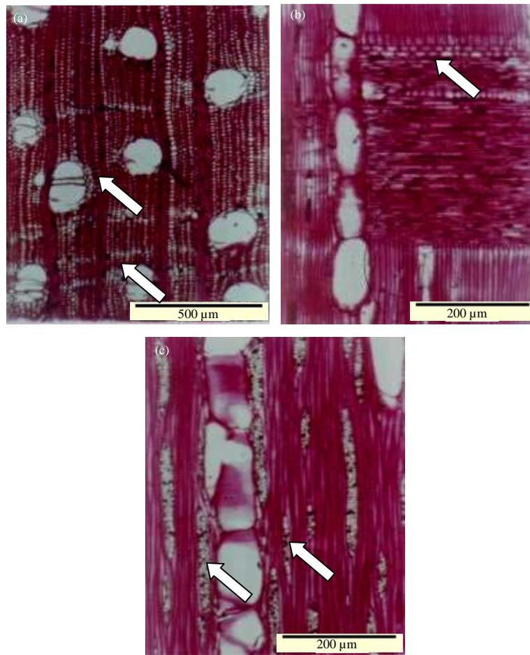
Fig. 6(a-c): *Cryptocarya aromatica* kostermans samples obtained from collection of the xylarium bogoriense 1915 bogor, Indonesia (40×magnification), (a) Transverse section: Axial parenchyma vasicentric and axial parenchyma bands 3-4 cells wide, (b) Radial section: Body ray cells procumbent with 3 rows of upright and square marginal cells and (c) Tangential section: (-2)-5 seriate rays
